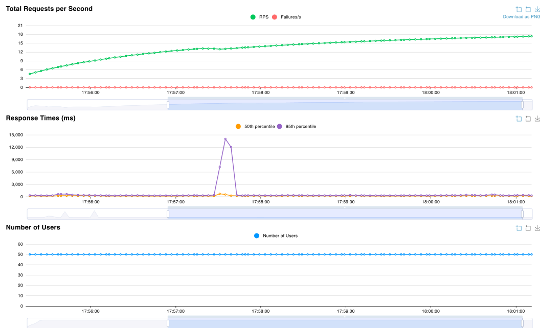
Figure 6: Locust live dashboard: requests per second, response-time percentiles, and active users
